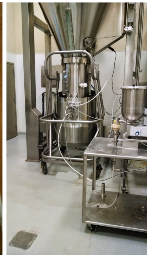
In-Process picture showing 18" wurster being fed with talc by a K-Tron powder feeder.
