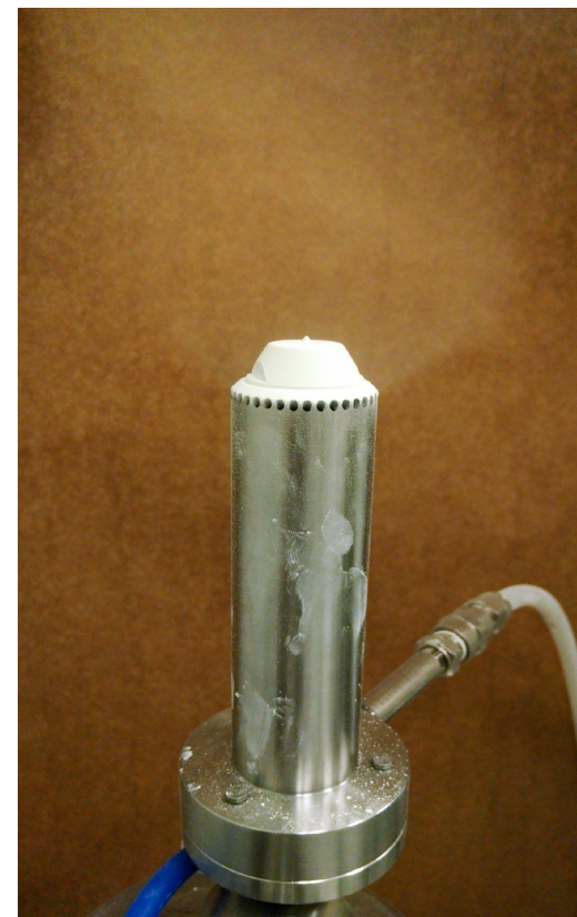
Modified Wurster Accelerator Sleeve with talc being delivered from the 45° air holes. Mounted on a standard Freund-Vector Wurster spray gun.
