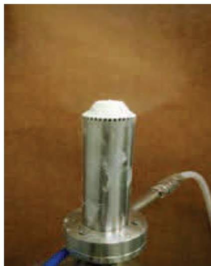
Diagram of a Freund-Vector Wurster coating system (Left) and a modified Wurster Accelerator spray gun with powder delivery capabilities (Right)
