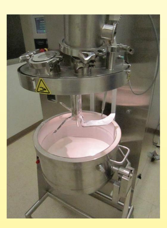
Samples of dry granulates were taken using a 5 ml sample thief at 6 and 10 minutes of mixing.
